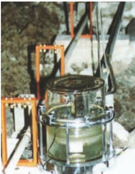
End and sensor of a 42m long water tube and a tiltmeter at the Geodynamic Station in Jameos del Agua which detect ground deformations
