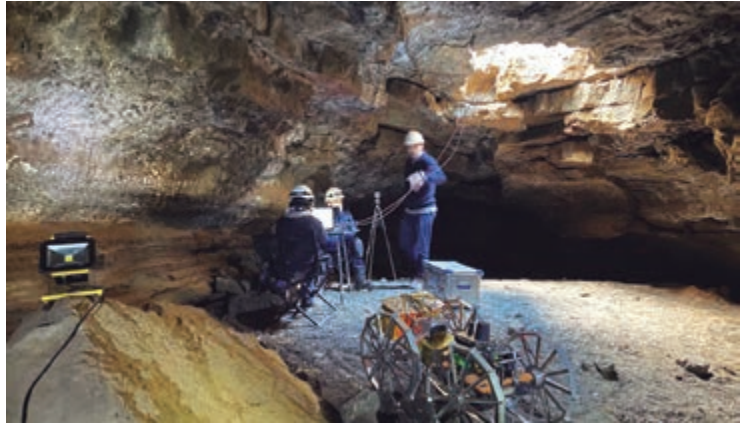
The underground laboratory at Cueva de los Verdes for geodetic monitoring of volcanic tremors, one of several such monitors which transmit their results to Madrid for assessment
